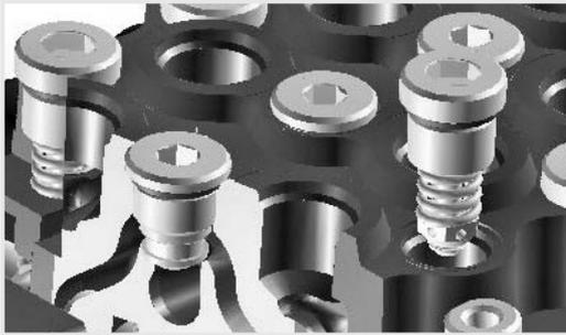
This picture shows the position of the auxiliary valves. For the tightening torque please see page 14.
