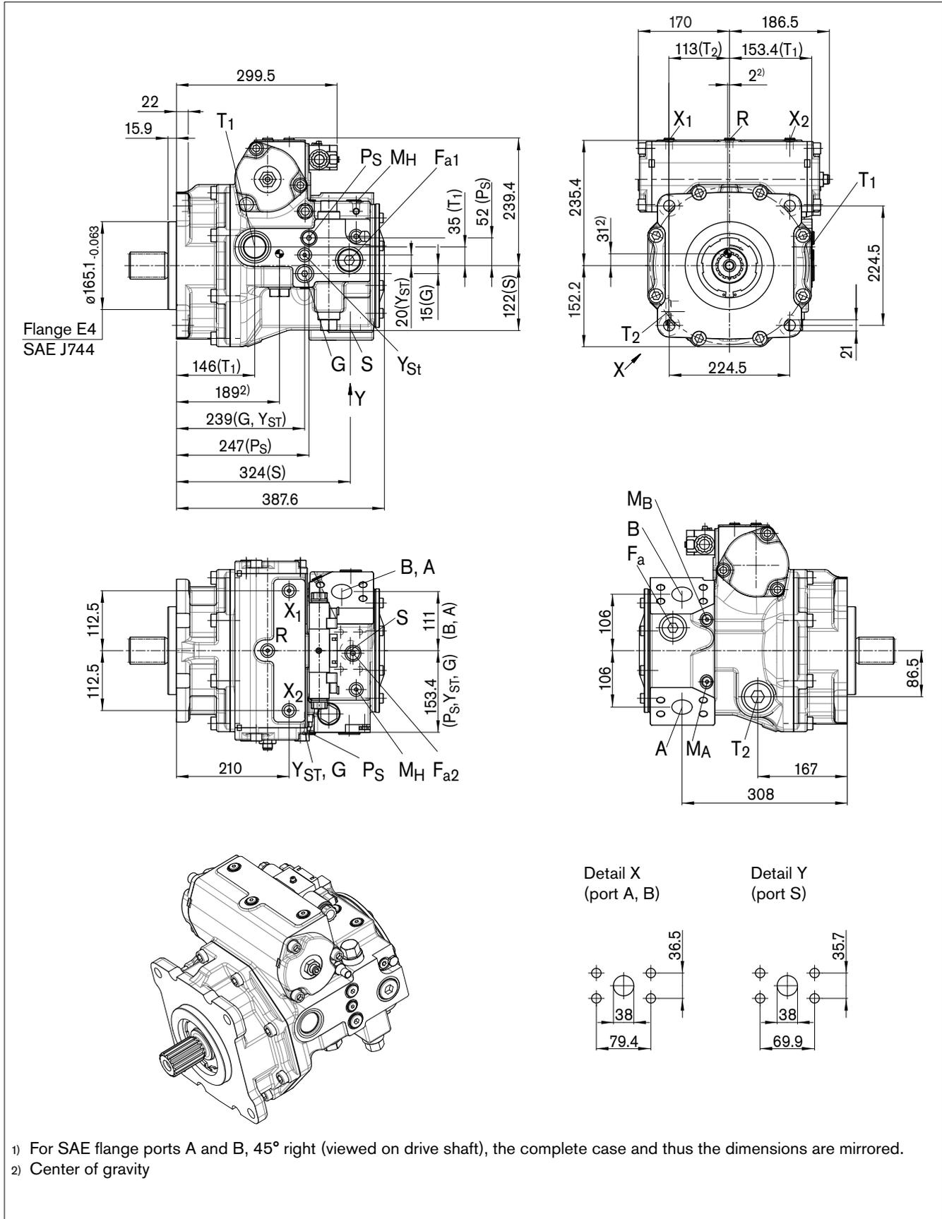
1) For SAE flange ports A and B, 45° right (viewed on drive shaft), the complete case and thus the dimensions are mirrored.
