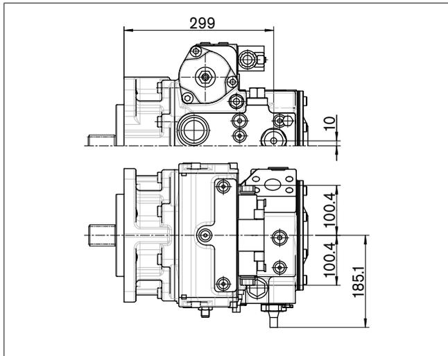
Version 4, 5 – valve fixed setting and inch valve mounted
