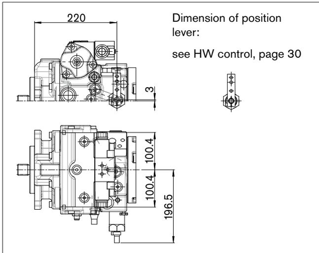
Before finalizing your design, request a binding installation drawing. Dimensions in mm.
