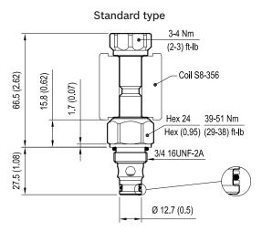
Version 4: Solenoid operated valve, poppet 2-way normally open
