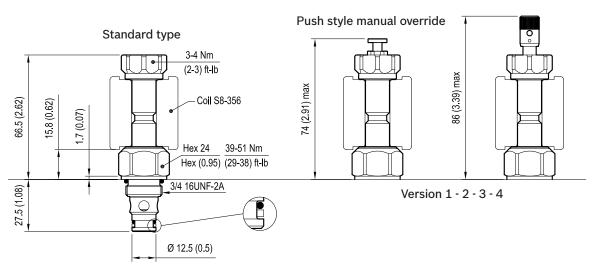
Version 2: Solenoid operated valve, poppet 2-way normally open Version 3: Solenoid operated valve, poppet 2-way double lock normally open
