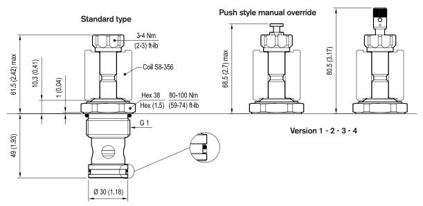
Version 2: Solenoid operated valve, poppet 2-way normally open
