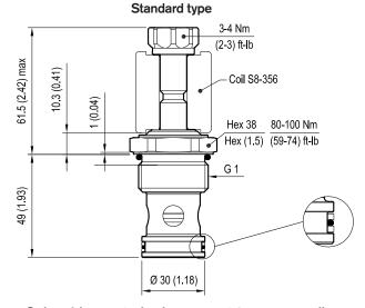
Version 4: Solenoid operated valve, poppet 2-way normally open
